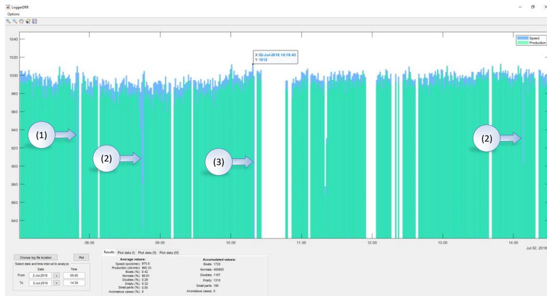
Figure 20. Instantaneous values of speed and production.
