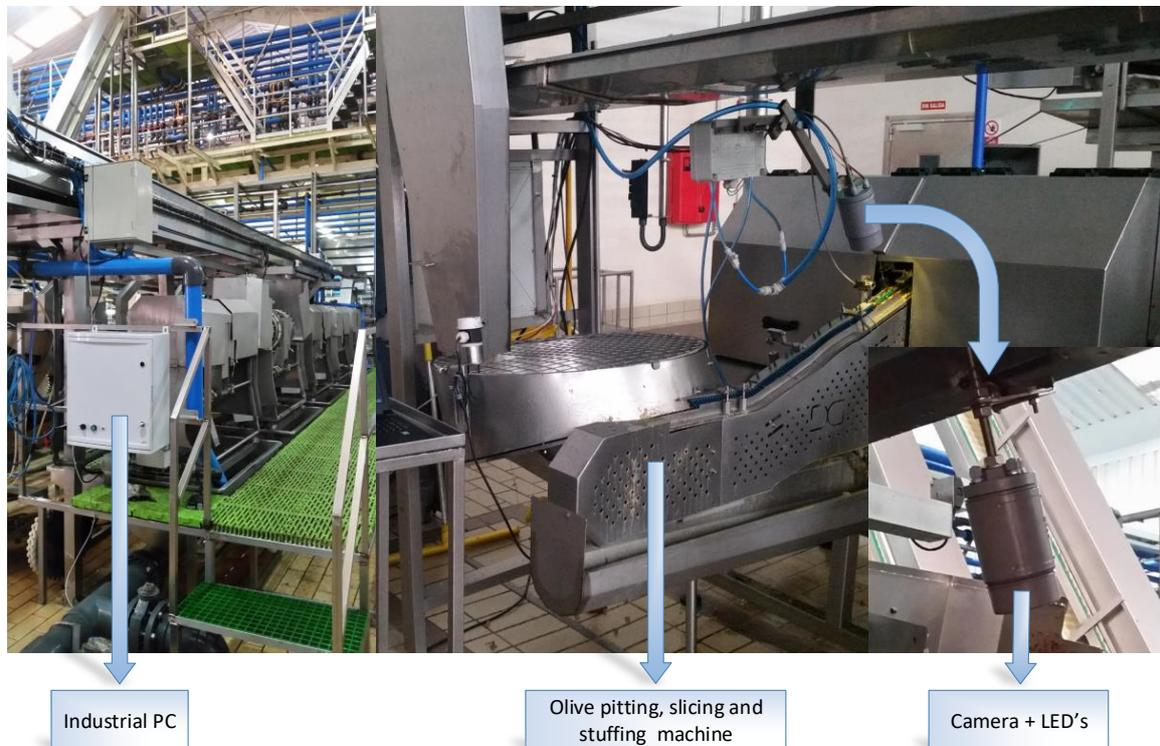
**Figure 9.** The system implemented on a “DRR machine”.
